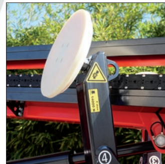
Stabiliser plates of a larger size to reduce the ground pressure.
