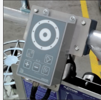
INTERCOM device for man-on-the-ground communication with personnel in aerial basket.
