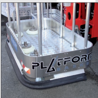
Anti-collision device in conductive rubber applied to the aerial basket.
